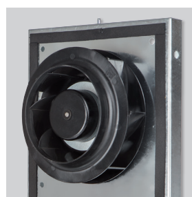
Backward impeller To prevent accumulation of dirtiness. Dynamically balanced. Plastic impeller for sizes 180 and 200, aluminium for 225 and 315A.
