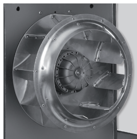
Centrifugal backward curved impeller To prevent accumulation of dirtiness. Dynamically balanced.
