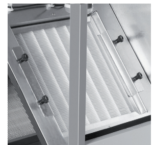
4 High-efficiency filters - Low pressure F7 filters (ePM1 70%) for supply air. - M5 filters (ePM10 50%) for extract air. Possibility of mounting a second filter inside the unit (accessory).
