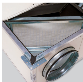
6 High-efficiency filters: - Low pressure F7 filters (ePM1 70%) for supply air. - M5 filters (ePM10 50%) for extract air. Possibility of mounting a second filter inside the unit (accessory).
