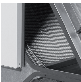
5 Counterflow heat exchanger high-efficiency (up to 93%), EUROVENT certified. All versions include internal bypass (approximately 75% over the nominal airflow).
