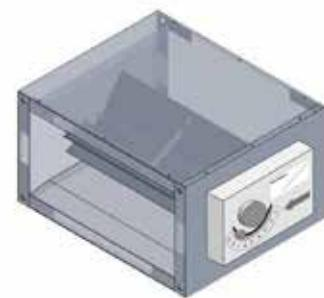
Constant volume flow regulators RPM-Q and RPM-Q-I are mechanical regulators used to maintain a constant volume flow rate independently of the pressure variations in ventilation and air conditioning systems. Regulators can be installed in a supply and extract air systems. Each regulator is set to the required flow rate and subjected to the aerodynamic function test conducted in our test facility.
