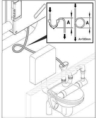
It is recommended to install the ALTAIR in the heated zone of the house. The minimum temperature should not be less than +10°C.
