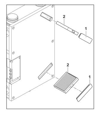
Everytime when filters are replaced the filter maintenance period has to be reseted pressing the button "A" during 5 seconds.
